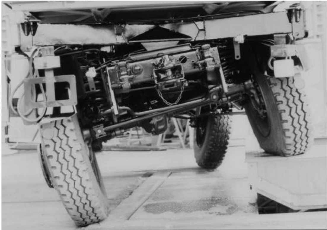
Figure 4.1 Chassis torsional flexion (induced in the RA only in this case)
